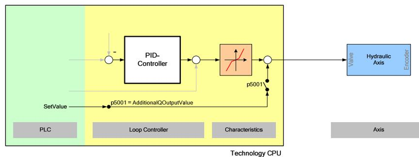
**Note** Before the superimposed output of the actuating variable for a hydraulic axis can be implemented via the p5000 parameter, the respective function must be activated via the p5001 parameter.
