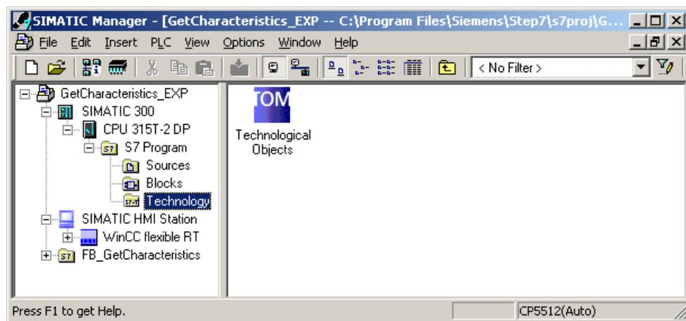
Check the suggested numbers of the technology data blocks and create the technology data blocks of the technology objects contained in the technology objects management by selecting the required objects and applying the “Create” button.
