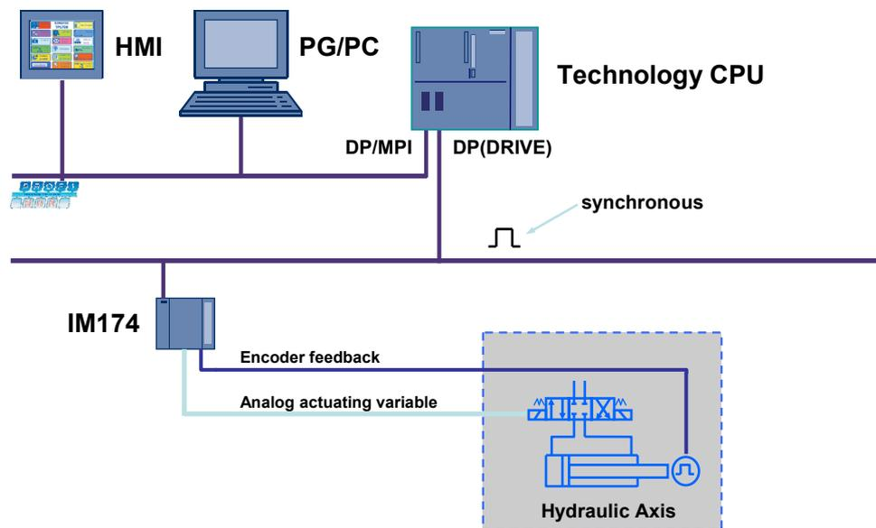
The interface module is connected via the DP (Drive) connection of the technology CPU, and it provides the necessary interfaces for the output of an analog setpoint value to the hydraulic valve, and for reading the encoder signal of the hydraulic axis or the hydraulic cylinder.
