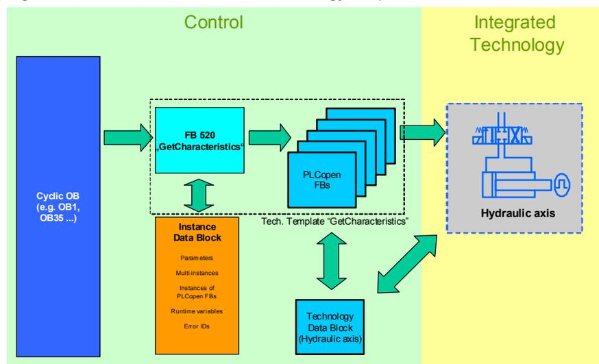
The technology object controlled by the FB 520 “GetCharacteristics” block is not allowed to be controlled by another part of the application program while FB 520 “GetCharacteristics” is active.
