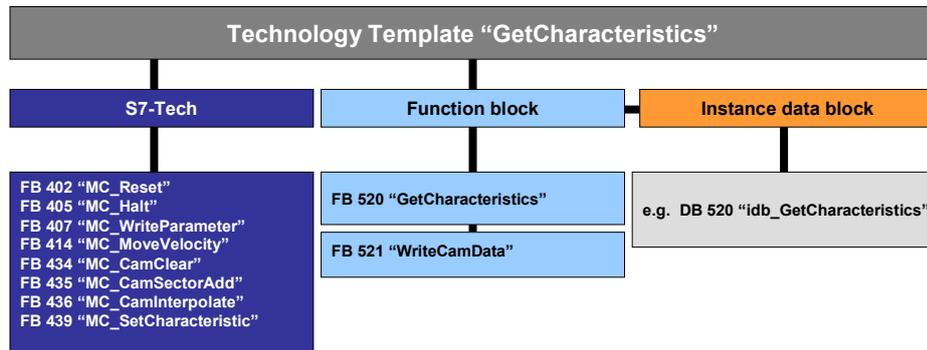
**FB 520 "GetCharacteristics"** contains the complete functionality for determining the compensation characteristic of a hydraulic axis. To do this, the function block performs measurements at the hydraulic axis in order to determine the compensation characteristic and saves this measured value in the instance data block of FB 520.
