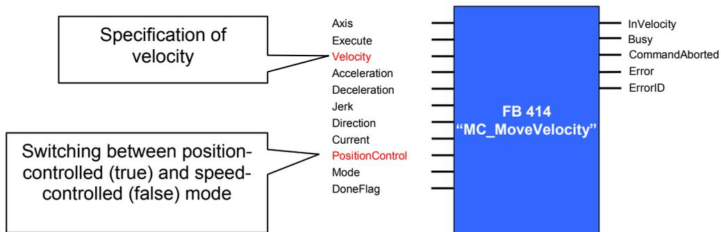
If the technology object is set to open-loop mode, the setpoint specification takes place only behind the controller. However, the hydraulic axis is still controlled via the compensation characteristic. This means that closed-loop control is disabled.
