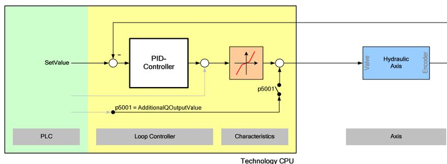
Via compensation characteristic, the linear behavior of the controller is, in the technology CPU, adapted to the non-linear behavior of the hydraulic axis.
