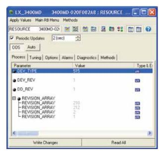
**Note:** Position 1 and 2 are scaled by 100. This means that 210 translates to rev 2.10, etc.
