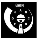
If the adjustable GAIN selector switch is set to "E" with the auto tune switch on, a Flowserve standard response tuning set will be calculated and used based on response parameters measured during the last RE-CAL.
