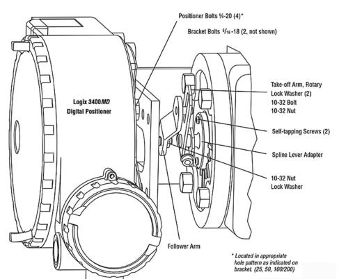
Figure 4: Standard Rotary Mounting
