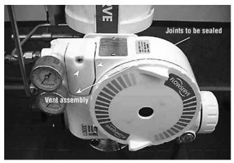
A small desiccant package as shown can be included under the sealing tape to ensure proper protection.
